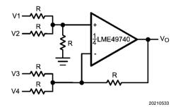
$V_0 = V1 + V2 - V3 - V4$
