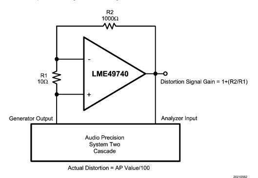
FIGURE 2. THD+N and IMD Distortion Test Circuit
