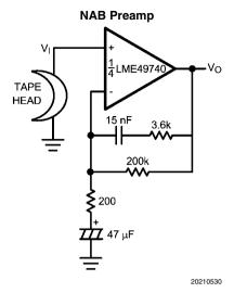
$A_V = 34.5$  F = 1 kHz  $E_n = 0.38 \text{ }\mu\text{V}$  A Weighted
